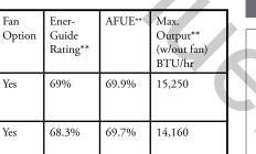
Rock \*\* EnerGuide Ratings and Outputs have been determined without a fan/blower, using the CSA P.4.1-02 test method
