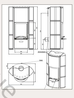
The body and face of the Etna, Elbrus, and Vesuv are made of high-grade steel in gray. They have a huge  $19'' \times 15\frac{1}{2}''$ fire window that glides effortlessly up and down via a silent counterweight system. A push-button finger latch releases the door outward for ease of cleaning.
