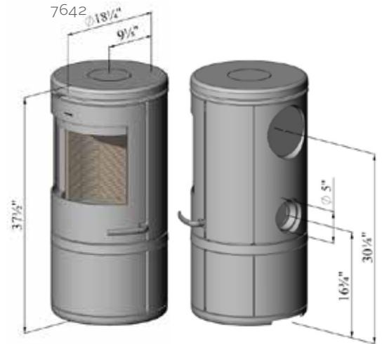
Basic Clearance (using single wall pipe top vent)
