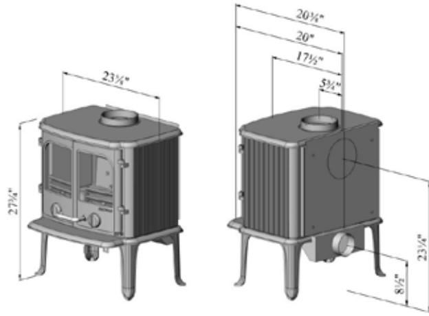
Basic Clearance (using single wall pipe top vent)
