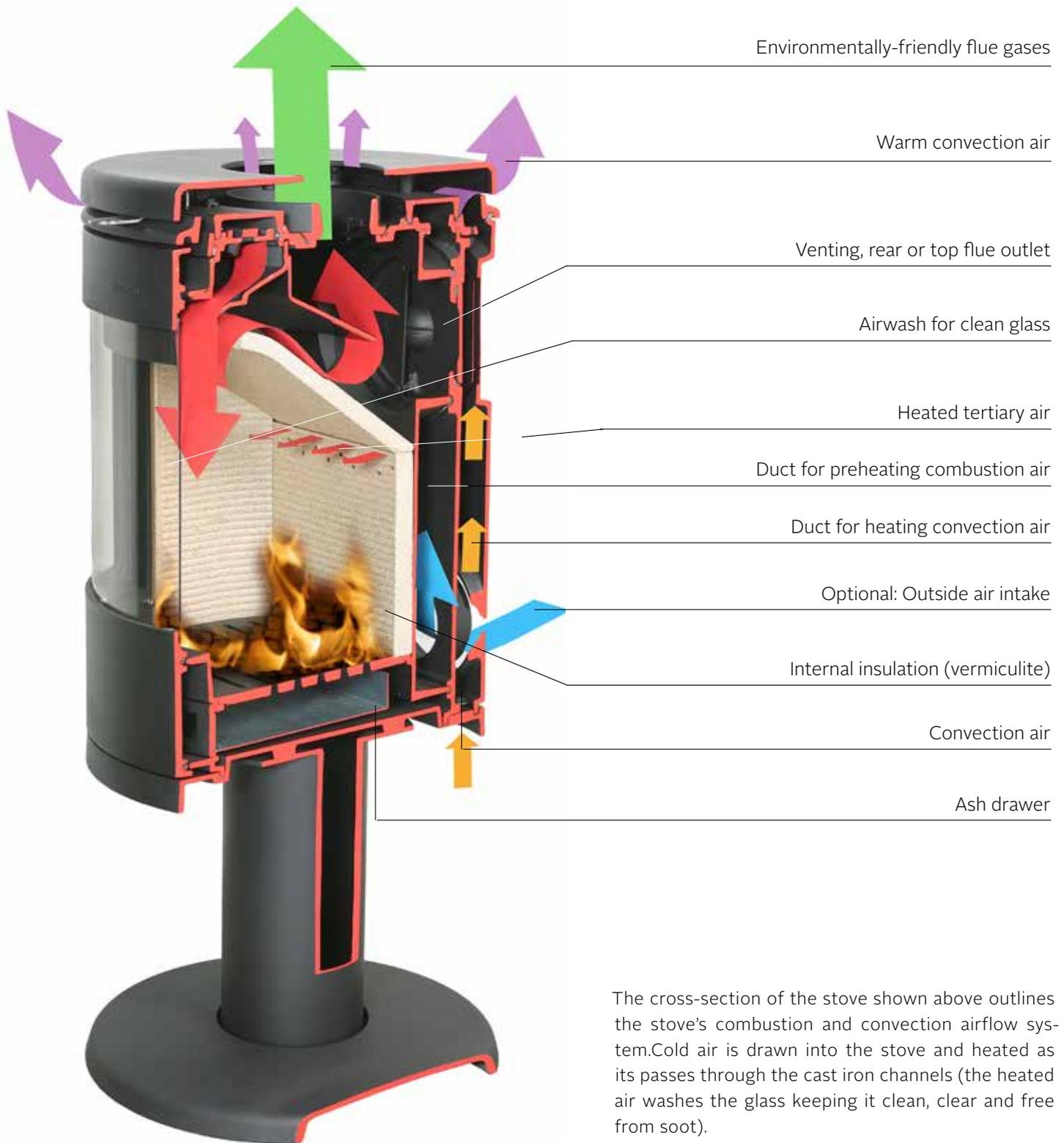
The cross-section of the stove shown above outlines the stove's combustion and convection airflow system. Cold air is drawn into the stove and heated as it passes through the cast iron channels (the heated air washes the glass keeping it clean, clear and free from soot).
