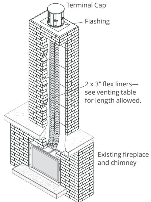
Note: The maximum vertical vent run for the Legend G4 is 40'. The minimum is 10'.
